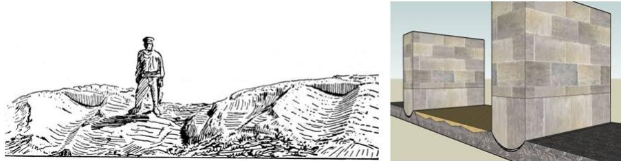
Figure 8. The rock foundations in the form of trough [Nauman, Arun, 2013]
