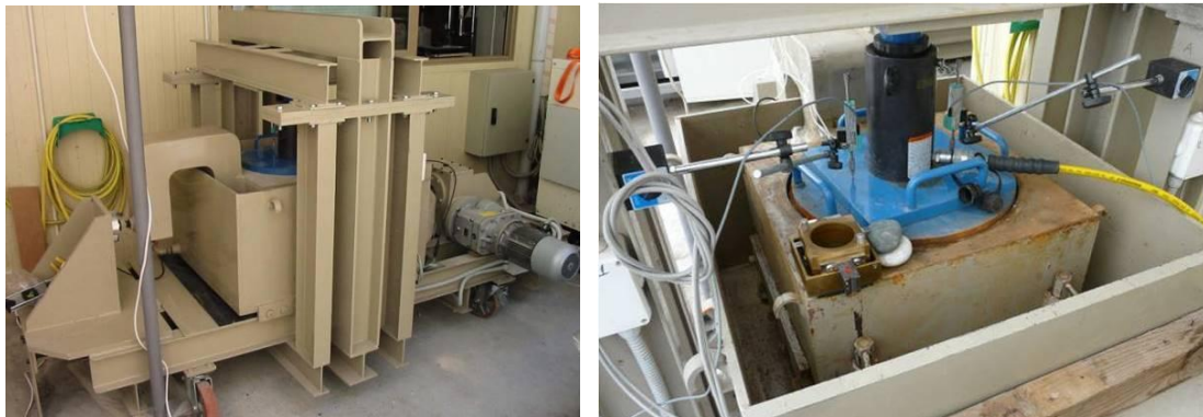
Figure 9. A schematic of the EDAFOS S.A. large-size direct shear device (top), and actual views of the large direct shear device: overall view (left), view of direct shear cell (right) -for comparison two cobbles of the largest size that may be included in the sample in this device and the cell of a conventional small-size direct shear device.
