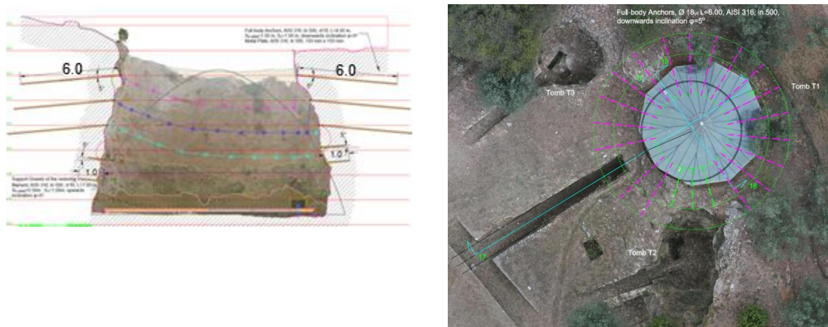
Figure 10. Arrangement of proposed measures for Tomb T1. Transverse Section S-18 (left) and Plan view of Tomb T1 (right). Excerpt from the Drawings of Structural Study (Egglezos, 2023).
