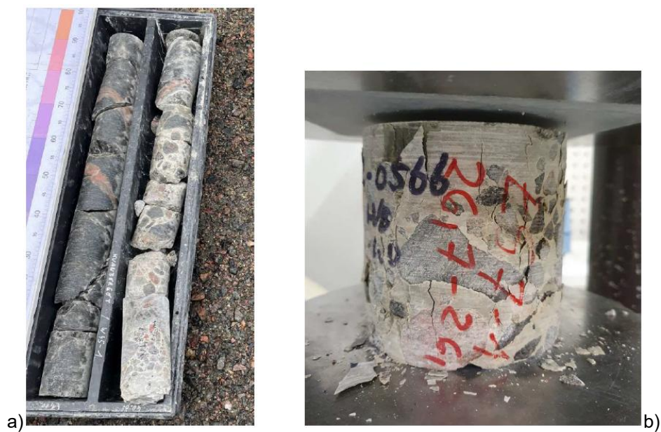
Figure 5. (a) Core samples from control drilling showing continuity of jet-grouted material; (b) specimen prepared for unconfined compressive strength testing.
