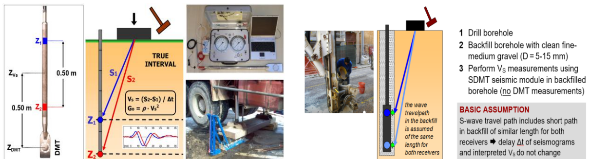
Figure 3. SDMT Test lay-out (left). V_s measurements by SDMT in backfilled boreholes in non-penetrable soils (right).
