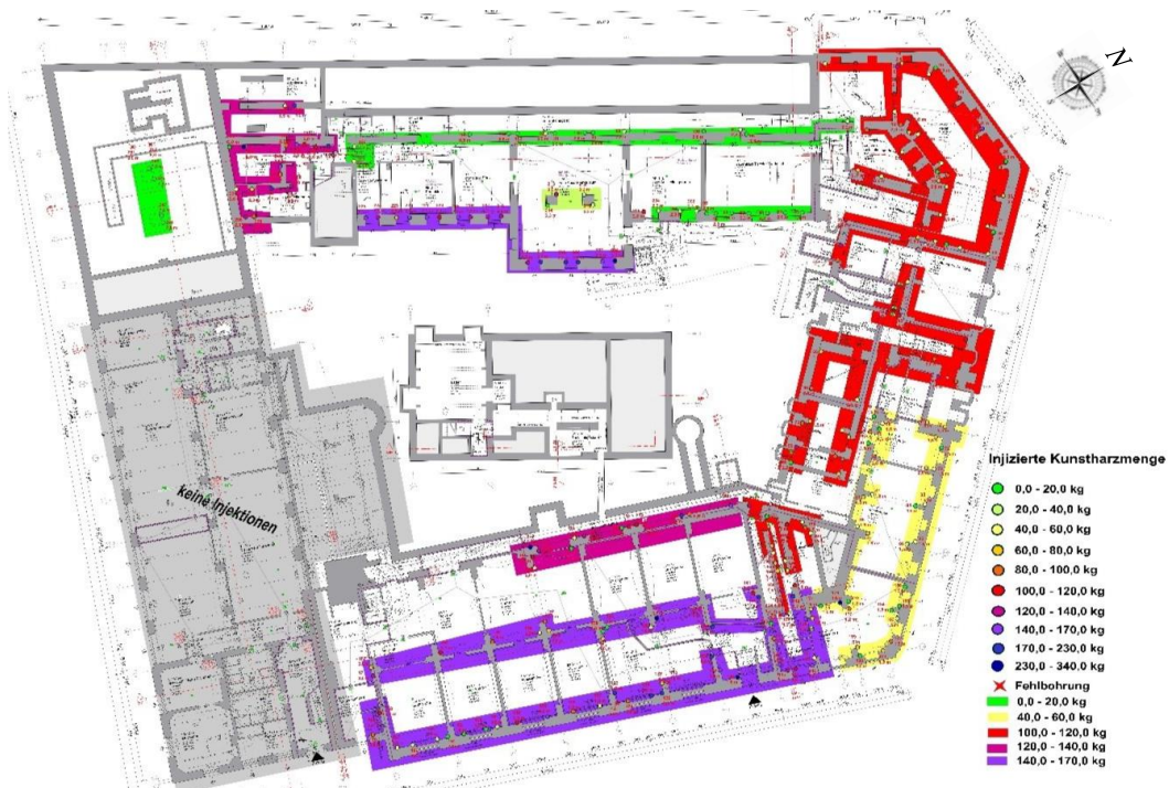
Figure 6. Overview of the building plan showing, for each treatment zone, the range of resin mass injected beneath the foundations and the corresponding resin mass per borehole
