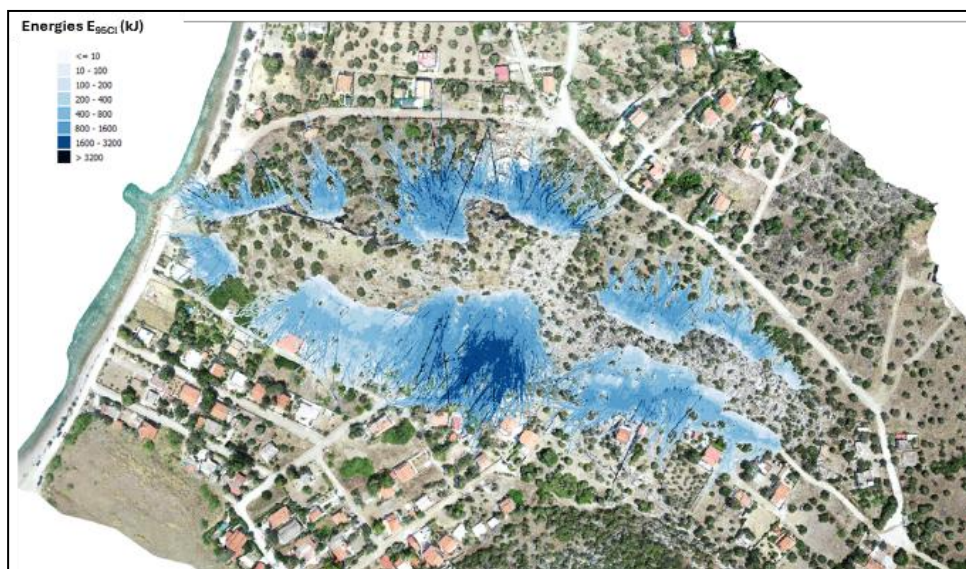
Figure 13. Distribution of kinetic Energies E_{95CI} in the surrounding area of the Acropolis of Voiotia.
