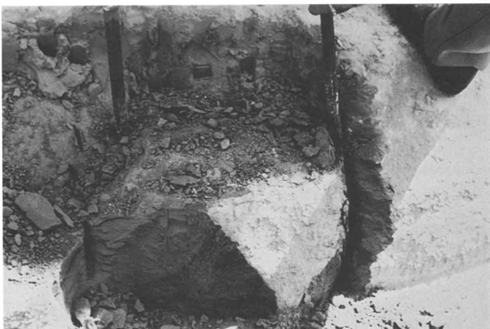
Fig. 10. Hand trimming of a block specimen
