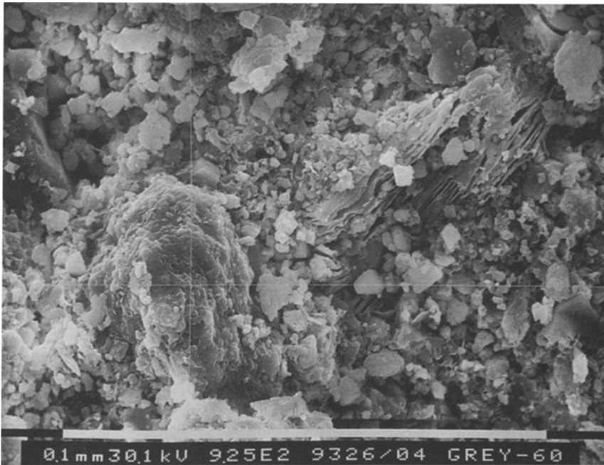
Fig. 4. s.e.m. microphoto showing platey clay minerals with a mica structure
